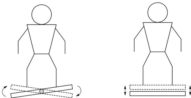
Figure 1 Different designs of whole body vibrating plates.
