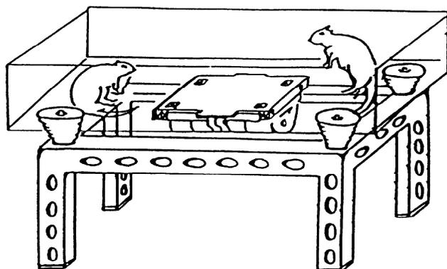
Fig. 1. Line drawing of the vibrating platform. An electric micro-vibrator (Micro 20TR,  $N = 22$  Watt,  $f = 50$  Hertz) is fixed under a metallic platform (45 cm/35 cm) over which a plastic cage of the same size is attached. The platform is lying on a metallic frame with 4 elastic vibrating cylinder placed at the 4 corners
